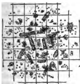
Microscopic Appearance of Common Calcined Magnesia.
